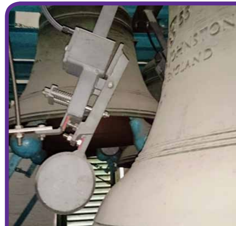
PHOTO 6 — Bell striking hammer mechanism for No. 7 Bell
